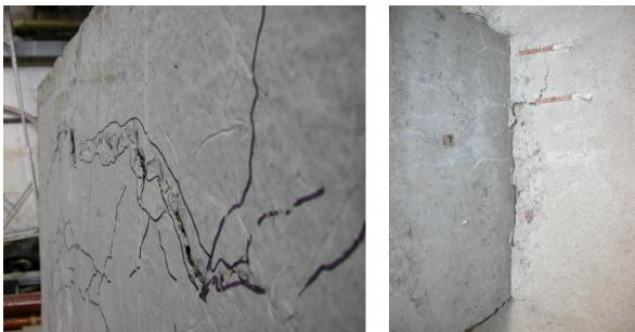
a) ring crack on the lower the slab face b) column cracks and spalls Figure 5. Cracks characterizing the punching pyramid
