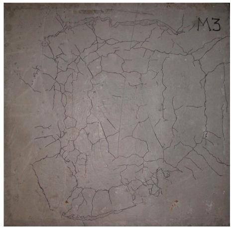
Figure 3. Lower (tension) slab face
